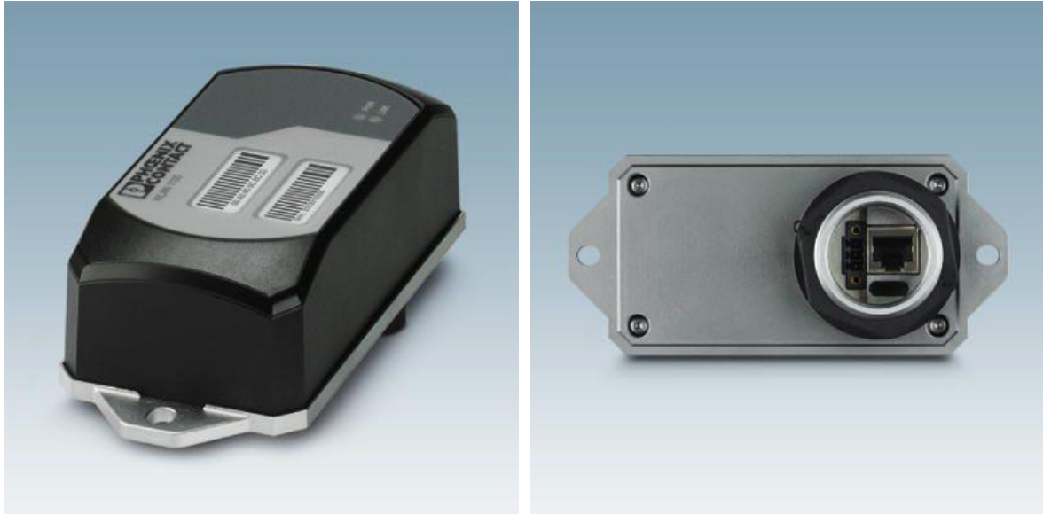
Figure 41 WLAN access point, client with two internal antennas (MIMO) for single-hole mounting, IP54, WLAN 802.11 a, b, g, n, frequency: 2.4 GHz, 5 GHz (incl. DFS channels), connections: COMBICON 9 ... 32 V DC, RJ45: for LAN, web, http/https, Command Line Interface
