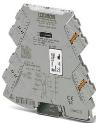
Figure 22 Limit value switch with changeover relay output for monitoring analog limit values from the sensor output. The sensor wash is activated at a mA value that corresponds to the limit value switch schedule with DIP switches activated. The relay closes or opens per user selection.
