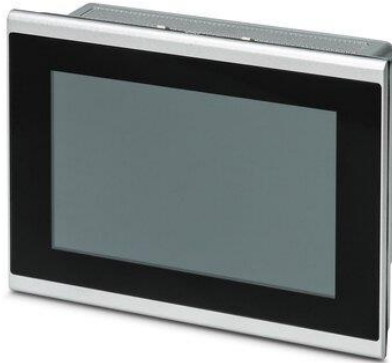
Figure 42 Panel mount external 7" touch display with connectivity of 4 sensors. Touch panel with 17.8 cm/7" TFT-display (Projective-capacitive (PCAP)), IP66 Touch panel with 7.0-inch widescreen (16:9) VGA, PCAP display, Software: Qt Browser
