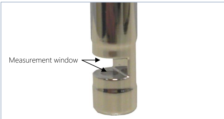
Fig.12: Measurement window on the sensor
