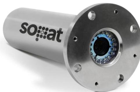
The InView system is equipped with a color camera and is suitable for many different particle detection tasks. The InView is equipped with a ring of LEDs, but additional LED panels can be used to illuminate the objects in different angles and distance. To reduce fouling on the InView window, we optionally provide a purging device which is mounted on the flange provided.
