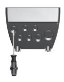
Pierce the pre-cut openings of the housing for as many cable glands as you wish to use and remove any remaining pieces from the openings.
