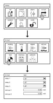
Set the mode to manual. Select the symbol TEST in the submenu IN/OUT.
