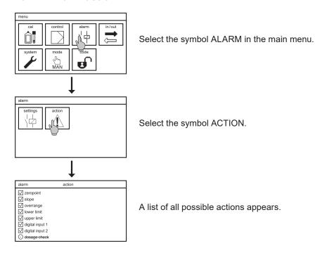
By activating the check boxes you can define actions as alarm actions. If a box is marked with a tick, the action or event will cause the alarm relay to switch. An empty box means that the action or event does not cause the alarm relay to switch. Overrange refers to both inputs, the message and alarm will occur if either input is affected.
