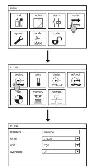
Select the symbol IN/OUT in the main menu and then the symbol ANALOG. A submenu opens, showing four drop-down lists.
