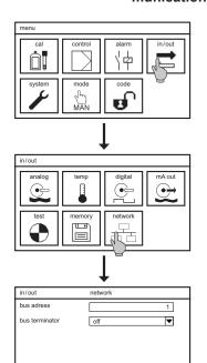
Select the symbol IN/OUT in the main menu and in the submenu, select the symbol NETWORK. Here you can set the following parameters:
