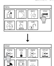
Select the symbol IN/OUT in the main menu, and in the submenu the symbol ANALOG. Subsequent to the usual parameters you find four more parameters that concern the cleaning function:
