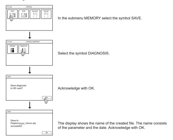
Note The .dia file is a binary file and can only be read with an appropriate configuration program.
