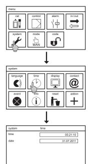
To set the internal clock, select the symbol SYSTEM in the main menu, and in the submenu the symbol TIME.
