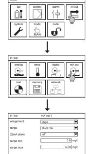
Select the symbol IN/OUT in the main menu and then select the symbol mA OUT. Here you can set the following parameters:
