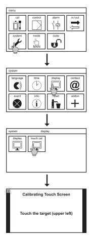
To calibrate the touch screen, select in submenu SYSTEM -> DISPLAY the symbol TOUCH CAL to start the calibration. The touch screen calibration texts are available in English only.
