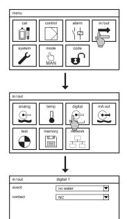
In the entry-level version, the Neon® instrument has one digital input. All settings concerning the digital input(s) are found in the submenu IN/OUT -> DIGITAL. If you have two digital inputs, separate symbols will appear for them.
