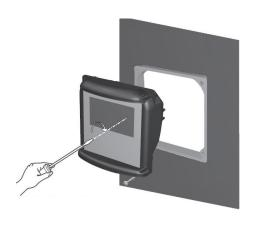
Place the instrument inside the frame and secure it with the M4 x 25 screws. Tighten the screws until the instrument is firmly fixed.
