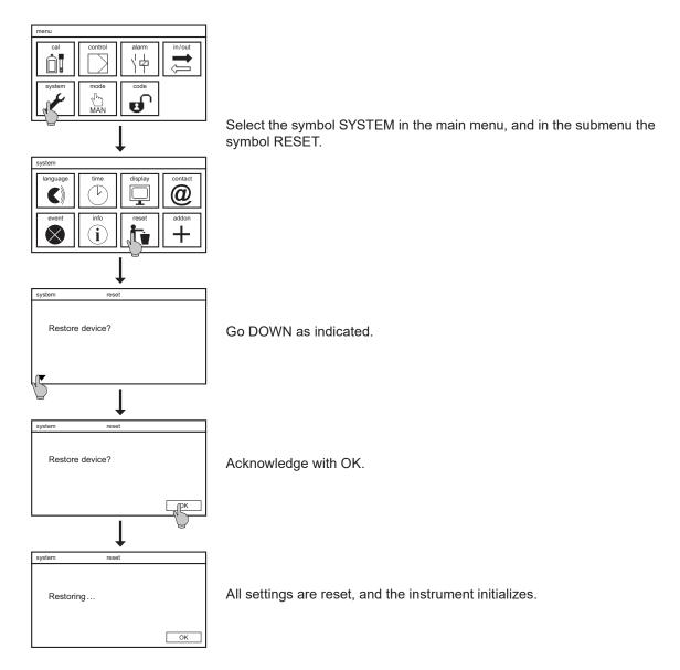
Note With touch screen instruments, the touch screen has to be calibrated after reset. The calibration routine starts automatically.
