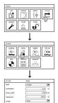
All settings concerning temperature measurement and compensation are found in the submenu IN/OUT -> TEMP. Select the symbol IN/OUT in the main menu, and TEMP in the submenu.
