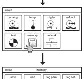
If the datalog add-on is activated, four symbols appear. In the menu LOG PARA you define which parameters you want to log. In LOG SET you define interval and log mode, and view the log status.
