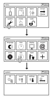
The submenu INFO is found in the submenu SYSTEM. It contains four symbols:
