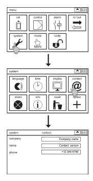
Select in the submenu SYSTEM the symbol CONTACT. For each field a keyboard opens to enter the name or number.
