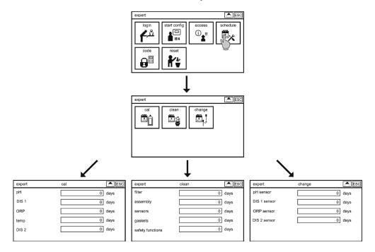
You can select an interval for each menu parameter. In this interval the maintenance message occurs. The message is shown until the user acknowledges.
