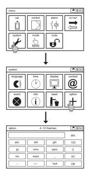
To activate add-ons, select the symbol SYSTEM in the main menu, and in the submenu the symbol ADD-ON.
