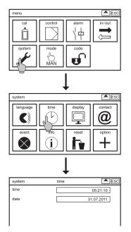
To set the internal clock, select the symbol SYSTEM in the main menu, and in the submenu the symbol TIME.
