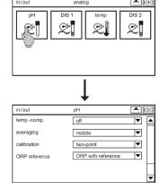
Choose in the main menu the symbol IN/OUT and in the submenu the symbol ANALOG and pH in the submenu.
