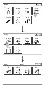
In the submenu ANALOG you can choose between the activated measuring inputs: pH, DIS 1, temperature, conductivity or DIS 2.
