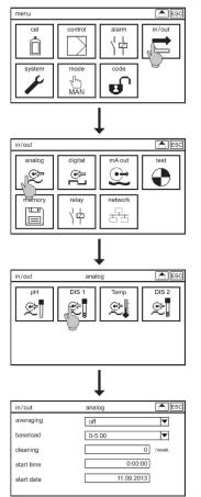
Select the symbol IN/OUT in the main menu, and in the submenu the symbol ANALOG, and then DIS 1. Subsequent to the usual parameters you find four more parameters that concern the cleaning function:
