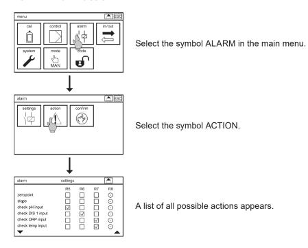
By activating the check boxes you can define which event should cause the alarm relays 5, 6, 7 or 8 to switch. An empty box means that the actions or event does not cause the relay to switch.
