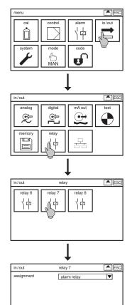
Select in the menu IN/OUT the symbol RELAY. In the submenu you can define for relays 6, 7 and 8 whether they work as alarm relays or have different functions.
