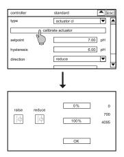
Besides set point, controller type, direction, p-range, integral time and differential time you can calibrate the actuator:
