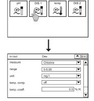
Select the symbol IN/OUT in the main menu, ANALOG in the submenu and then DES.
