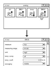
Select the symbol IN/OUT in the main menu, ANALOG in the submenu, and DIS 2 in the submenu.
