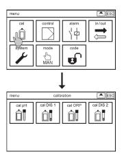
Select the symbol CAL to enter the submenu CALIBRATION and select the parameter for calibration.
