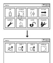
In the main menu select the symbol CONTROL. In the CONTROL menu you find the following submenus: pH, DIS 1, and optionally EC or DIS 2, in which you define parameters for control and output.
