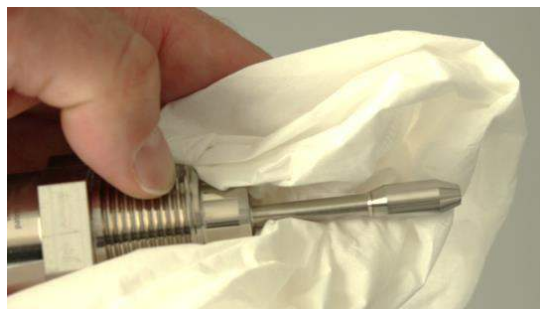
Cleaning the sensor with solvent-saturated cloth or paper
